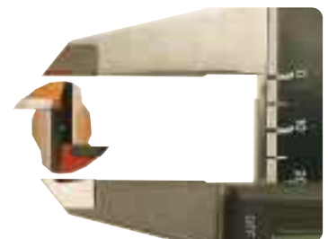
Notice the space created when measuring the diameter from the cutting edge (left) and from the body of the bit (right). This little space makes a big difference in the efficiency of chip and sawdust ejection.
